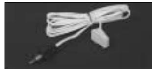
ter marked with a double wave. The water alarm sensor is suitable for nearly all fluids. Stick the sensor with the supplied double-sided adhesive tape to the wall so that the contacts touch the floor. The signal is triggered as soon as both contacts are wetted by the fluid.
